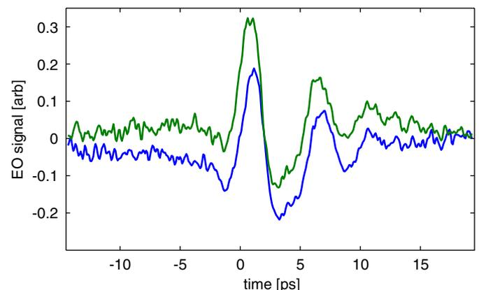
Fig. 4. The electro-optic signal of the CSR emitted from the entrance to the dipole magnet. Two separate measurements are shown to demonstrate the level of reproducibility.
