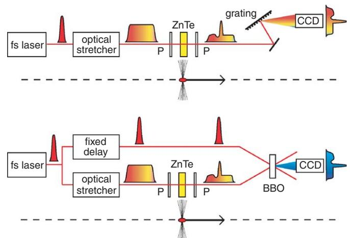
Fig. 2. The general layout for the techniques of spectral decoding (top), and temporal decoding (bottom). Only the ZnTe crystal is within the beamline.
