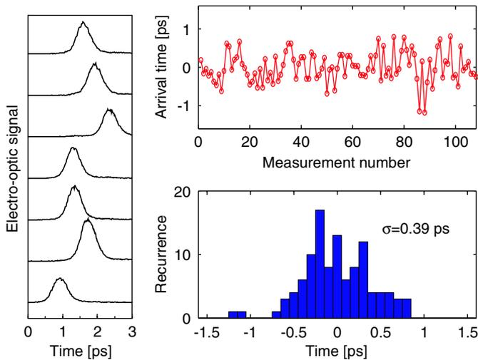
Fig. 3. A series of single-shot temporal decoding measurements of FELIX electron bunches (50 MeV, 300 pC), showing the timing jitter between the laser and electron bunch. The rms timing jitter of 390 fs is comparable to the bunch length of 275 fs rms (650 fs FWHM) [3].
