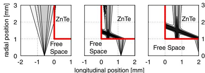
Fig. 1. The Coulomb field of a low  $\gamma$  electron as it passes a dielectric slab. The contours are for field scaled by radial position,  $r^2 E_{\text{Coulomb}}$ . The field outside the crystal region is as calculated in the absence of the crystal.
