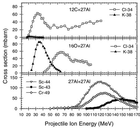
FIG. 2. Cross sections for the production of  $^{34}\text{Cl}$ ,  $^{38}\text{K}$ ,  $^{49}\text{Cr}$ ,  $^{43}\text{Sc}$ , and  $^{44}\text{Sc}$  calculated using the PACE-2 evaporation code for [ $^{12}\text{C} + ^{27}\text{Al}$ ], [ $^{16}\text{O} + ^{27}\text{Al}$ ], and [ $^{27}\text{Al} + ^{27}\text{Al}$ ] compound nucleus formation.
