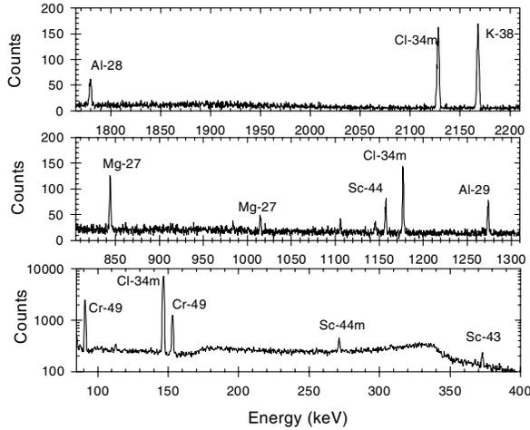
FIG. 1. Gamma-ray spectrum in an aluminum activation sample after irradiation with ions from an aluminum target foil.  $^{34m}\text{Cl}$ ,  $^{38}\text{K}$ ,  $^{28}\text{Al}$ ,  $^{29}\text{Al}$ ,  $^{24}\text{Na}$ ,  $^{27}\text{Mg}$ ,  $^{49}\text{Cr}$ ,  $^{43}\text{Sc}$ ,  $^{44}\text{Sc}$ , and  $^{44m}\text{Sc}$  peaks are observed.
