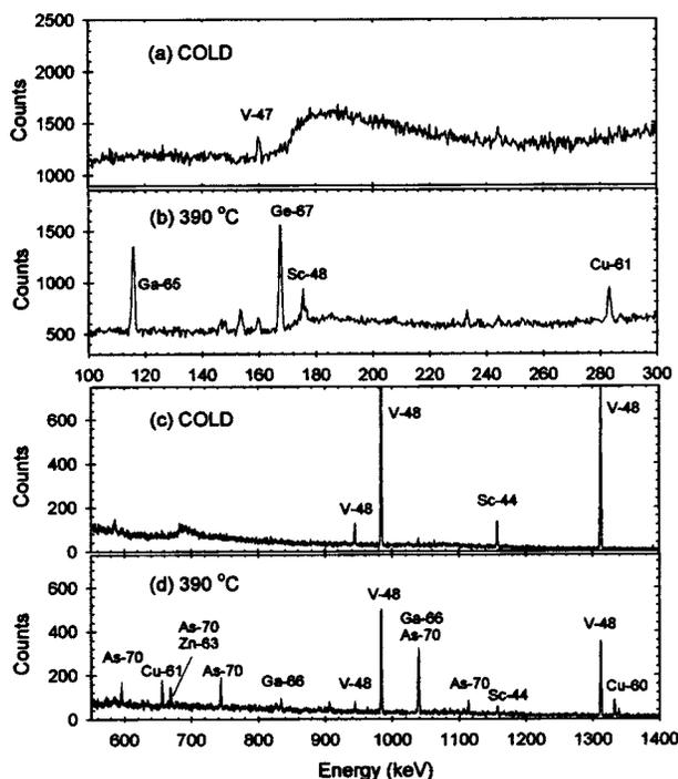
FIG. 1. Gamma-ray spectra observed in a Ti activation sample after irradiation with ions from a primary aluminum target foil which was (a), (c) unheated and (b), (d) heated to 390 °C.
