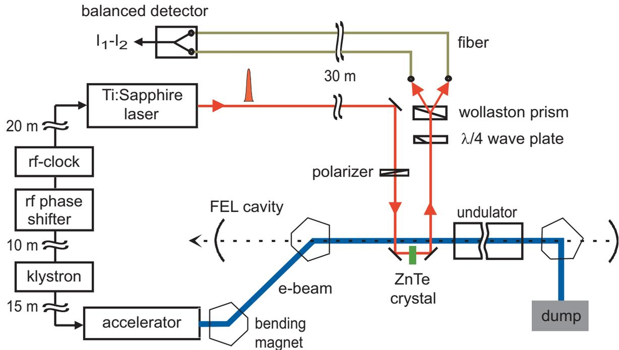
Figure 1: Experimental setup of the electro-optic "delay-scan method".
