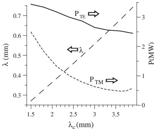
Fig. 3. Wavelength and output peak power of the TE wave, as well as output peak power of the TM wave versus the magnetic field (measured in wavelengths).
