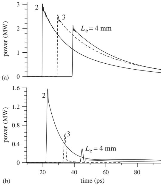
Fig. 2. Output power of the TE (a) and the TM (b) waves versus the time at various e-bunch lengths.
