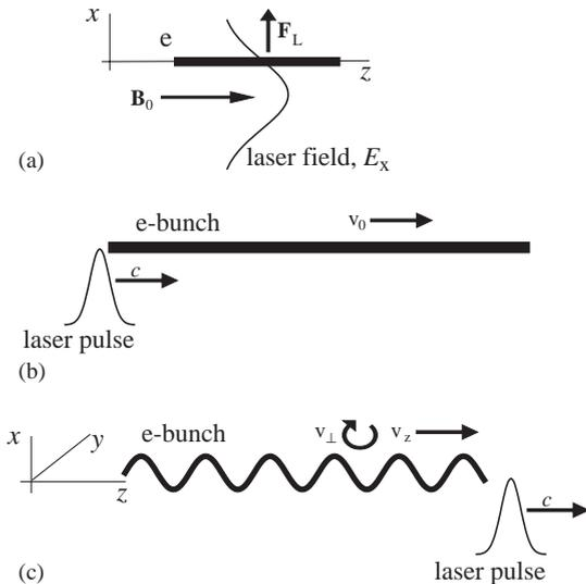
Fig. 1. Ponderomotive force provided by the laser pulse (a), and e-bunch before (b) and following (c) laser kicking.
