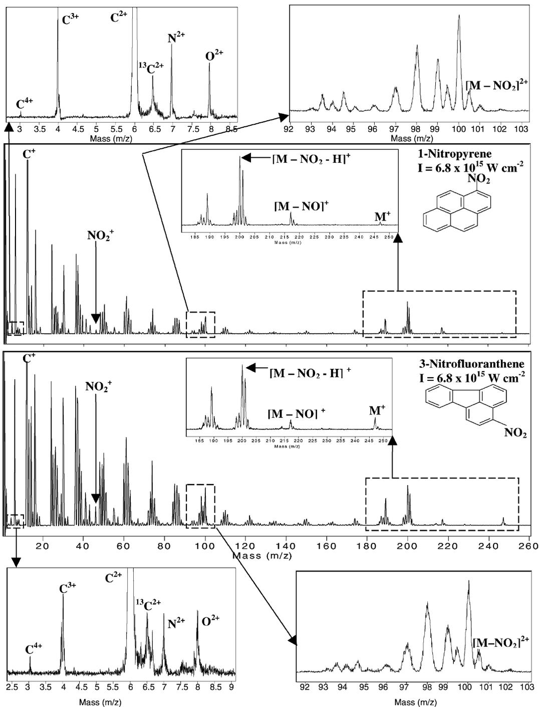
Fig. 9. A comparison of femtosecond mass spectra of 1-nitropyrene and 3-nitrofluoranthene. Both molecules have a mass of 247 Da but their structures differ significantly.
