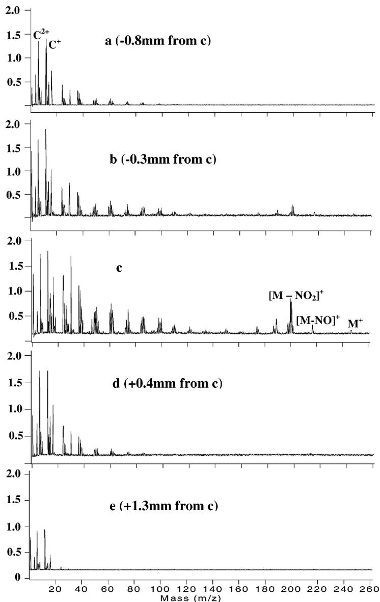
Fig. 11. Mass spectra of 1-nitropyrene recorded using varying positions of the focussed beam in the y-axis (i.e., perpendicular to the time-of-flight axis and the plane of propagation of the beam).  $I = 4 \times 10^{15} \text{ W cm}^{-2}$ .
