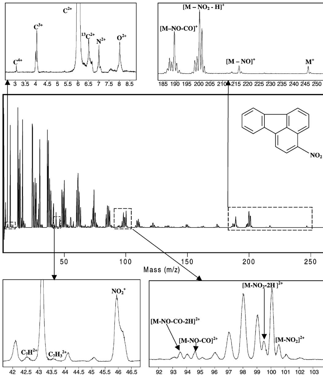
Fig. 6. Femtosecond mass spectrum of 3-nitrofluoranthene;  $\lambda = 800$  nm,  $I = 1.0 \times 10^{16}$  W cm $^{-2}$ .
