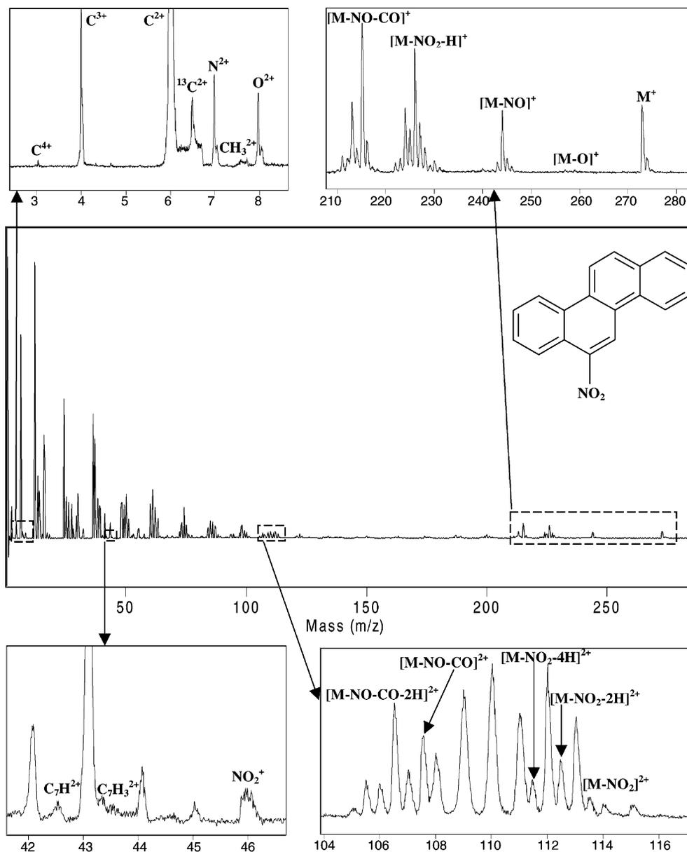
Fig. 7. Femtosecond mass spectrum of 6-nitrochrysene;  $\lambda = 800$  nm,  $I = 1.1 \times 10^{16}$  W cm $^{-2}$ .
