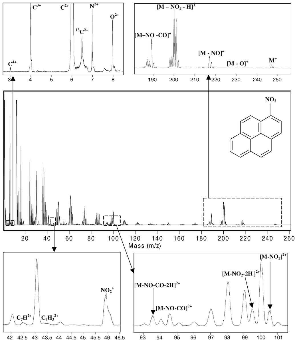
Fig. 5. Femtosecond mass spectrum of 1-nitropyrene;  $\lambda = 800 \text{ nm}$ ,  $I = 6.8 \times 10^{15} \text{ W cm}^{-2}$ .
