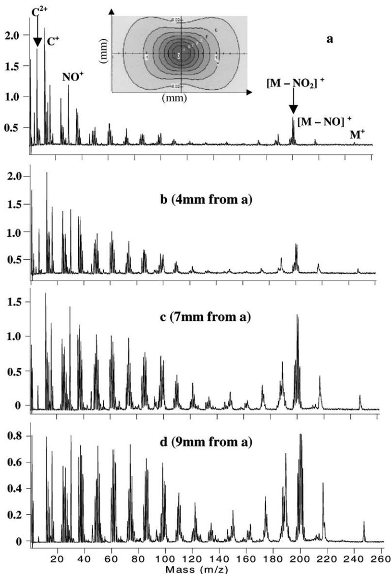
Fig. 10. Mass spectra of 1-nitropyrene recorded at an intensity of  $4 \times 10^{15} \text{ W cm}^{-2}$ . The spectra were taken using varying positions of the focussed beam (in the plane of propagation of the beam). The inset shows the typical intensity contours for a focused Gaussian pulse of varying intensities.
