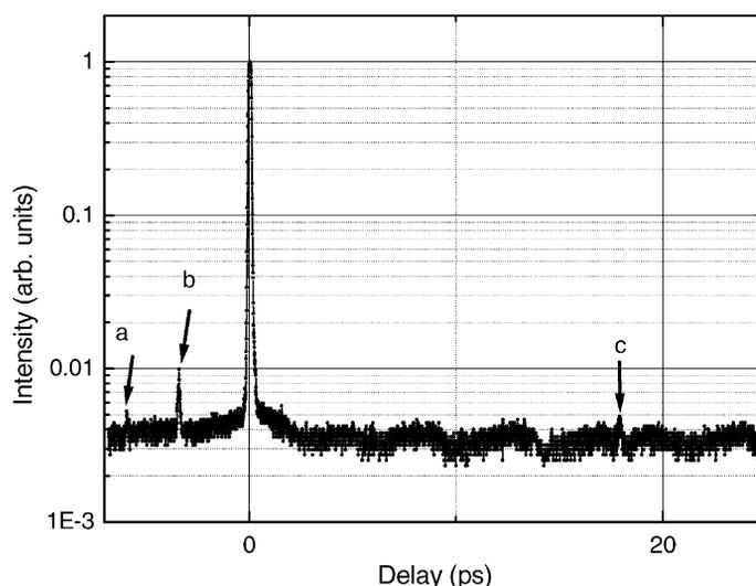
Fig. 1. Cross correlation of 800 nm laser pulse containing the following features: (a) pre-pulse at the rate of  $-5.97$  ps; (b) reflection from SHG crystal at the rate of  $-3.39$  ps; (c) post-pulse at the rate of  $17.9$  ps.
