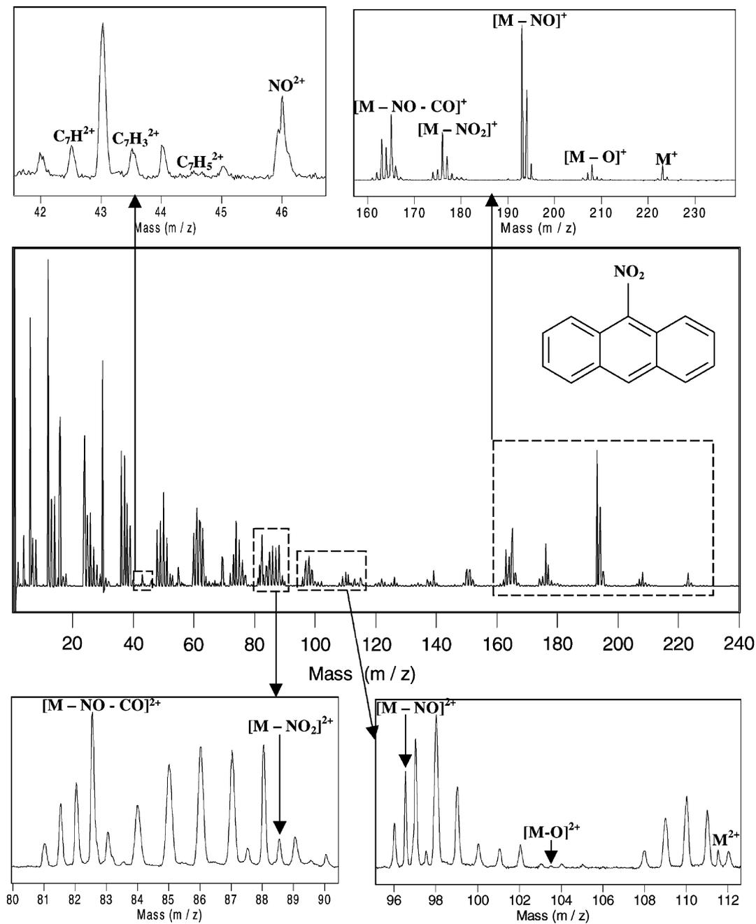
Fig. 3. Femtosecond mass spectrum of 9-nitroanthracene;  $\lambda = 800$  nm,  $I = 2.5 \times 10^{15}$  W cm $^{-2}$ .
