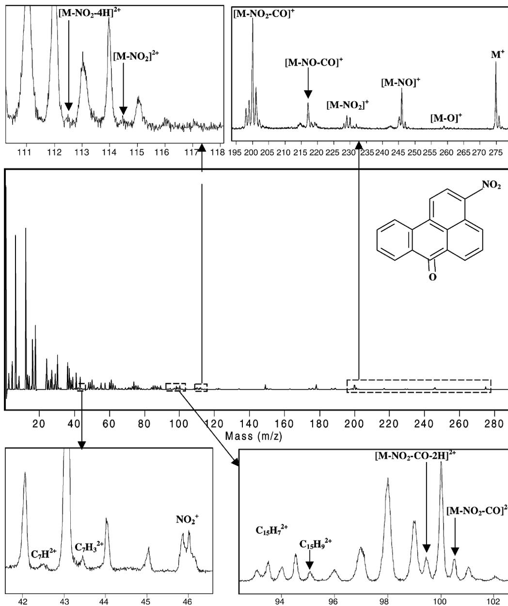
Fig. 8. Femtosecond mass spectrum of 3-nitrobenzanthrone;  $\lambda = 800\text{ nm}$ ,  $I = 1.3 \times 10^{16}\text{ W cm}^{-2}$ .
