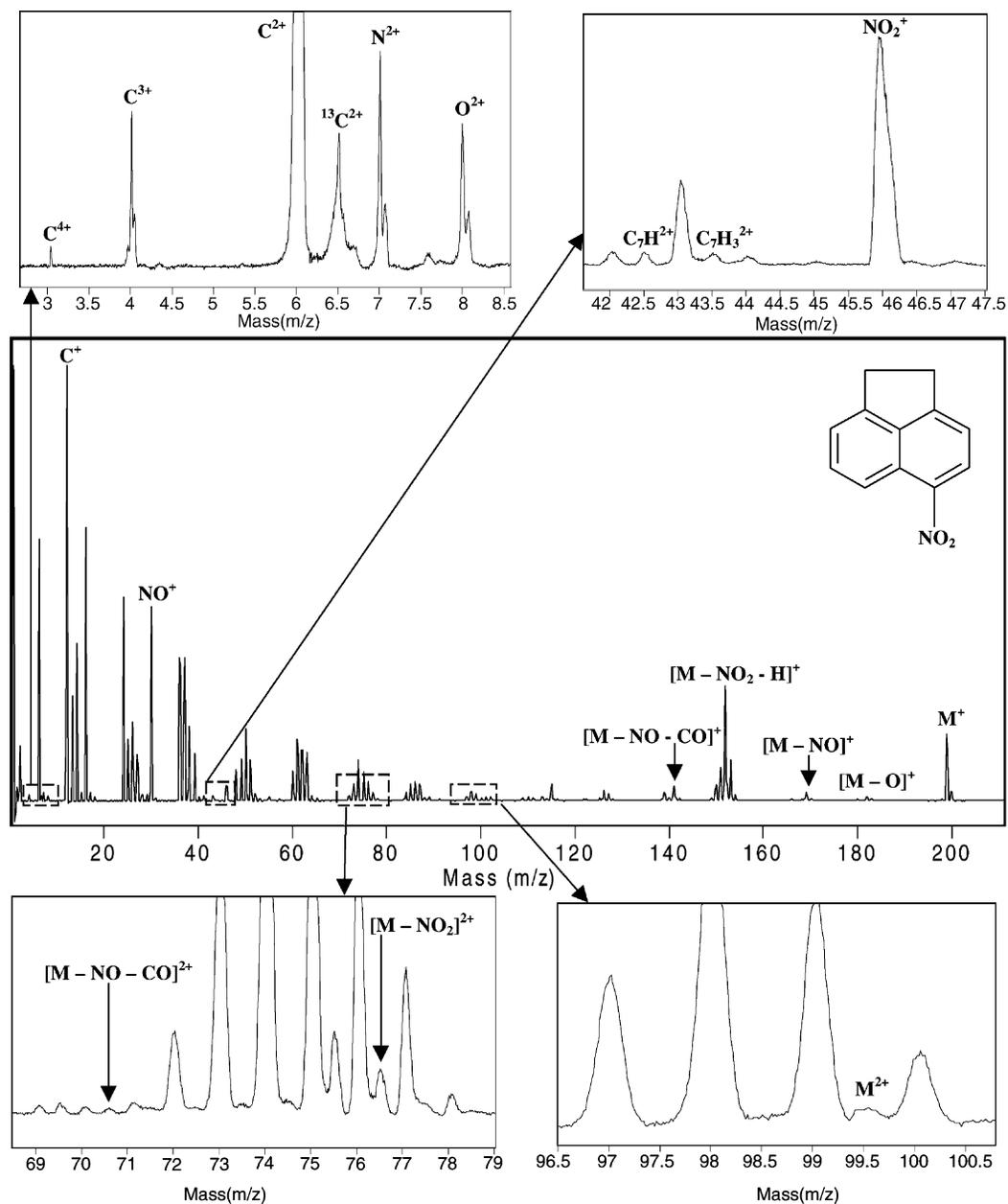
Fig. 4. Femtosecond mass spectrum of 5-nitroacenaphthene;  $\lambda = 800$  nm,  $I = 1.3 \times 10^{16}$  W cm $^{-2}$ .
